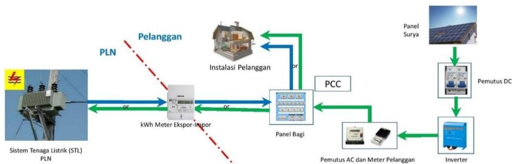
**Gambar 2. Solar Home System On Grid**
