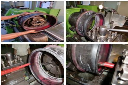
Gambar 7. Proses machining cylinder transition (Sumber : PT PJB UP Gresik, 2015)
