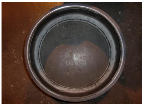
Gambar 8. Hasil machining cylinder transition (Sumber : PT PJB UP Gresik, 2015)
