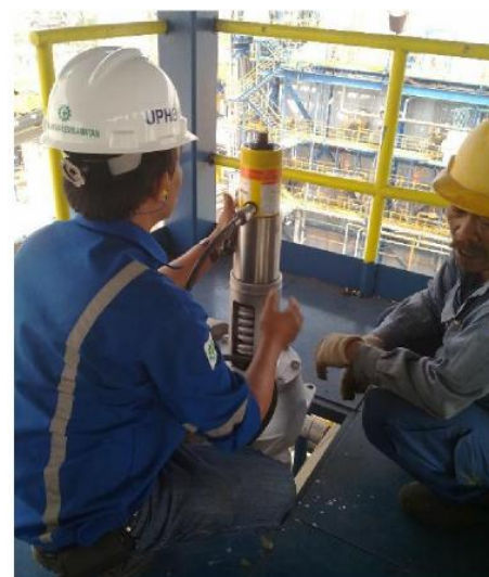
Gambar 13. Pengetesan safety valve
