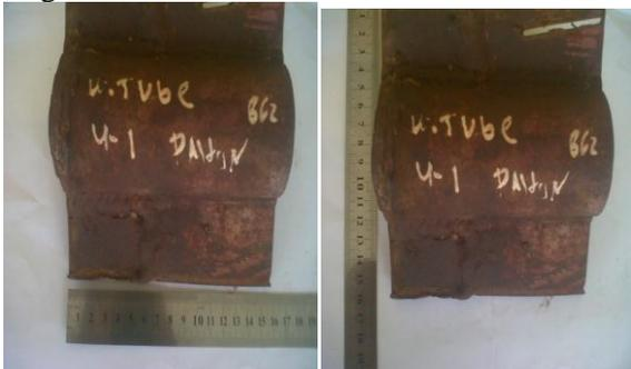
Gambar 12. Waterwall tube boiler ASTM SA178D
