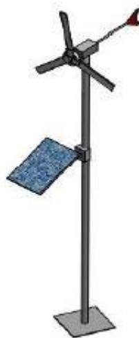
**Gambar 1.** Desain Hybrid One Pole Energy
