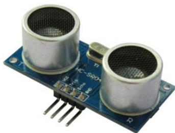
Gambar 1. Sensor Ultrasonik
