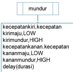
Gambar 9. Flowchart Gerak Robot 4
