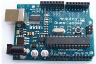
Gambar 1. Board arduino ATmega328
