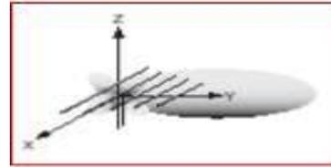
Gambar 2. Pola radiasi antenna yagi
