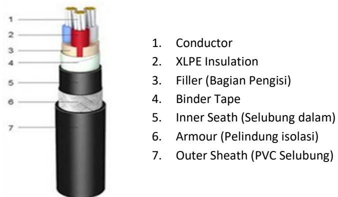
Gambar 3. Penampang Kabel XLPE ( indonesian.alibaba.com )
