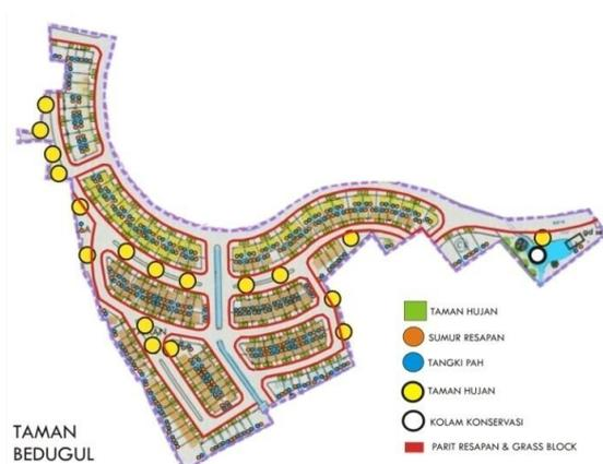
Gambar 15. Usulan Desain Perletakan Konsep *Zero Runoff*
