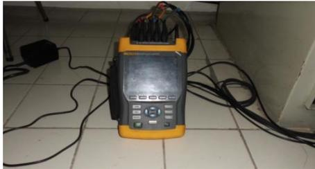
Gambar 8. Alat ukur *Power Analyzer* Fluke 435
