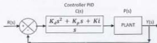
Gambar 3.2 Kontrol *Proportional Integral Differential*
