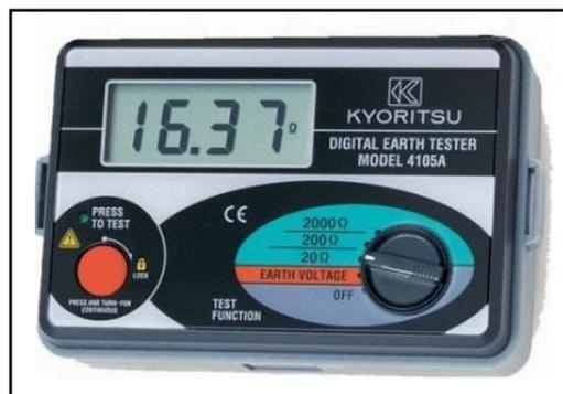
Gambar 4. alat ukur pentanahan digital
